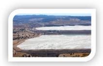
dissolves silver and gold particles. The gold and silver laden solution is then collected and treated in a process that extracts the gold and silver. Gold/silver bullion is then produced for sale to the open market. Once the ore is processed the contaminated waste pile must be managed in accordance with Federal and State regulations, which requires regulated storage and monitoring.
